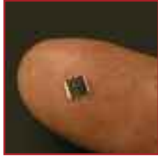
active surface of a triple junction cell: 3x3 mm
