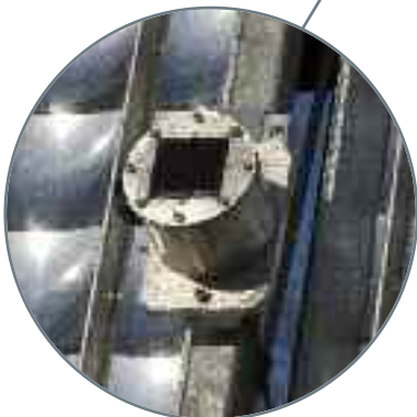
Solar camera (part of the overall tracking system)
